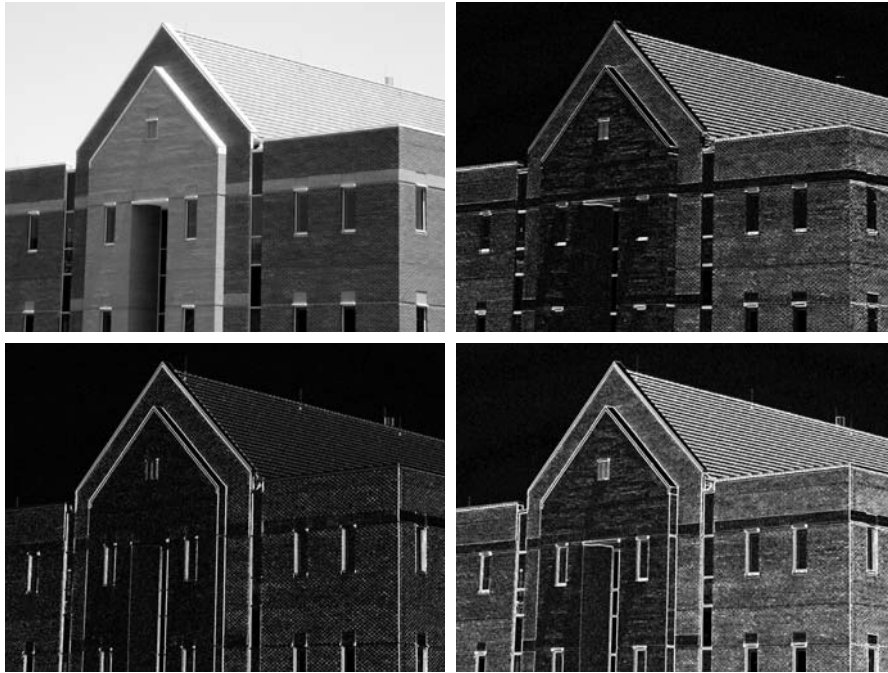
FIGURE 10.16 (a) Original image of size 834 \times 1114 pixels, with intensity values scaled to the range [0, 1] . (b) |g_x| , the component of the gradient in the x -direction, obtained using the Sobel mask in Fig. 10.14(f) to filter the image. (c) |g_y| , obtained using the mask in Fig. 10.14(g). (d) The gradient image, |g_x| + |g_y| .
