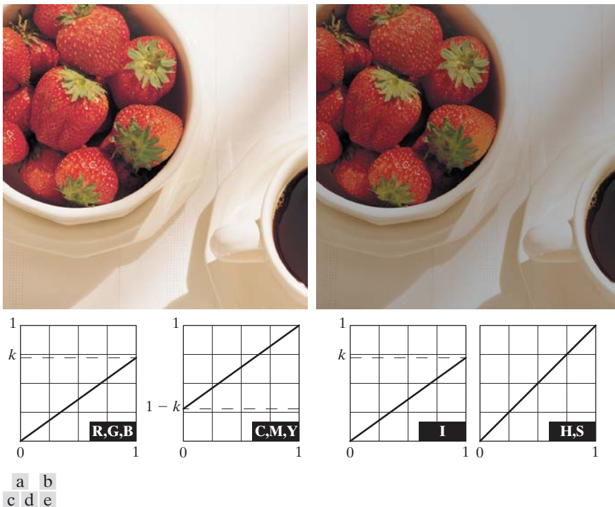
FIGURE 6.31 Adjusting the intensity of an image using color transformations. (a) Original image. (b) Result of decreasing its intensity by 30% (i.e., letting k = 0.7 ). (c)–(e) The required RGB, CMY, and HSI transformation functions. (Original image courtesy of MedData Interactive.)
