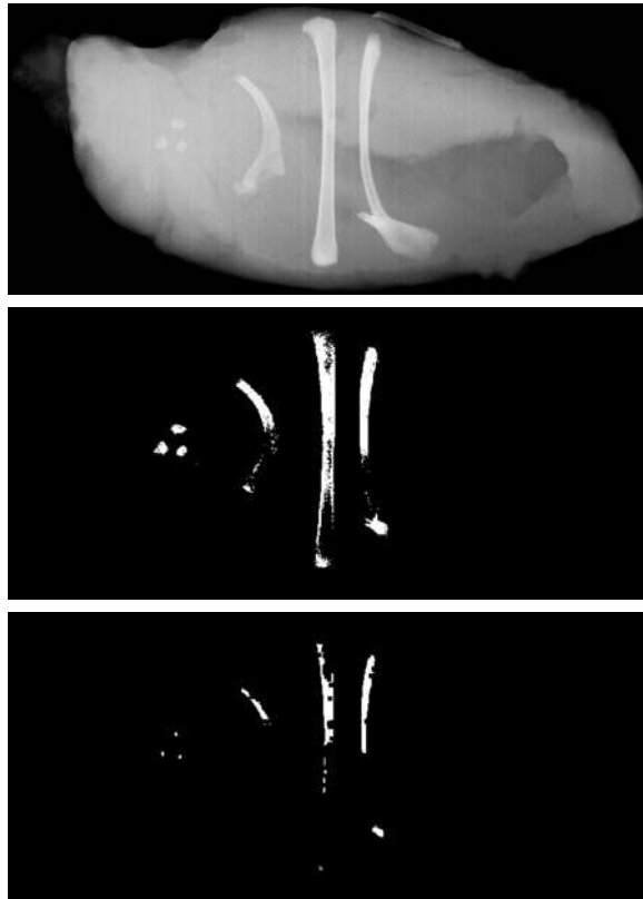
FIGURE 9.18 (a) X-ray image of chicken filet with bone fragments. (b) Thresholded image. (c) Image eroded with a 5 \times 5 structuring element of 1s. (d) Number of pixels in the connected components of (c). (Image courtesy of NTB Elektronische Geraete GmbH, Diepholz, Germany, www.ntbxray.com .)
