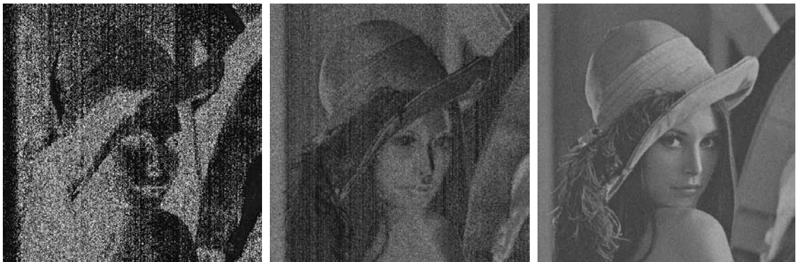
FIGURE 6.49 HSI components of the noisy color image in Fig. 6.48(d). (a) Hue. (b) Saturation. (c) Intensity.
